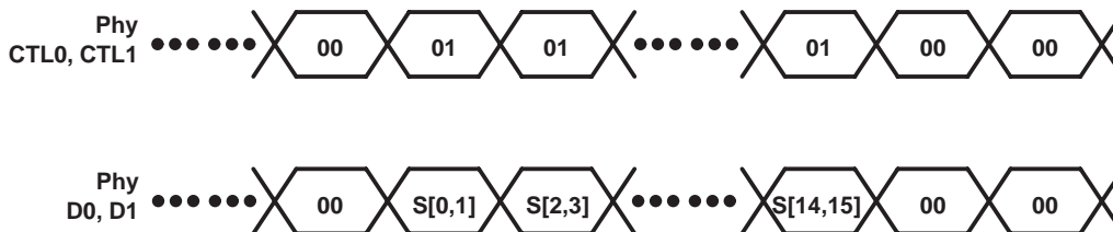
Figure 6. Status Transfer Timing
